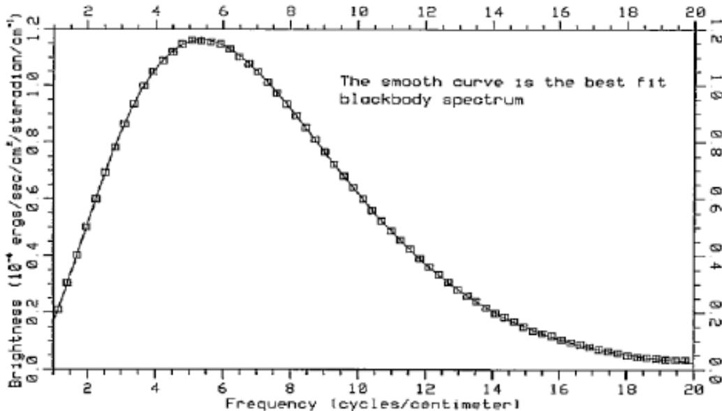
Figure 5: The CMB frequency spectrum as measured by the FIRAS instrument on the COBE satellite [3]. This first spectrum from FIRAS is based on just 9 minutes of measurements. The CMB temperature estimated from it was  $T = 2.735 \pm 0.060$  K. The final result from FIRAS is  $T = 2.725 \pm 0.002$  K (95% confidence) [4]. Using data from other experiments as well, the best current value is  $T_0 = 2.72548 \pm 0.00057$  K (68% confidence) [5].
